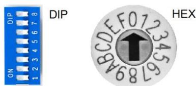
Fig. 4.1. View of the toggle switches
